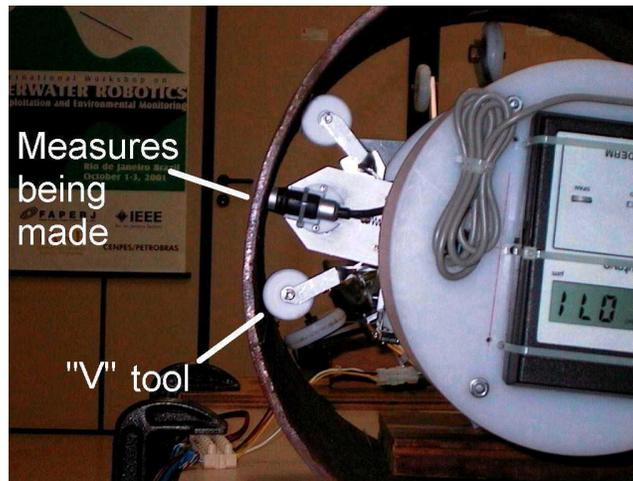
Figure 3. SIMCRODUTO operation and the "V" tool (with two side-wheels).
