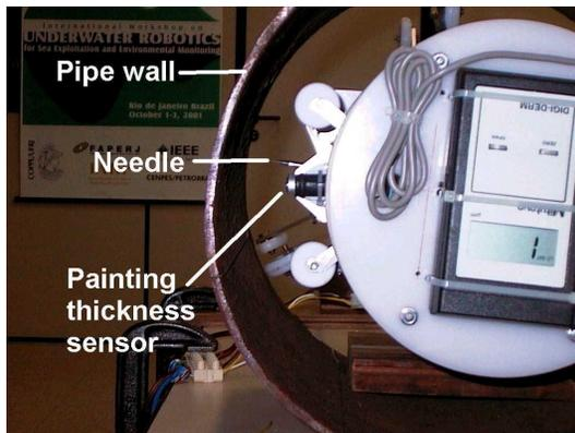
Figure 1. SIMCRODUTO: Detail of the painting thickness sensor and the tactile sensor (needle).
