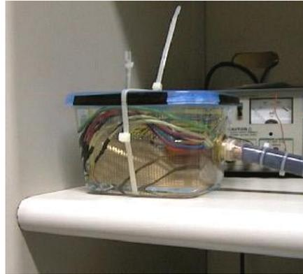
Figure 5. Circuit inside thin-wall plastic housing filled with silicon oil.
