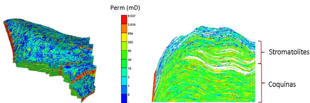
**Figure 2.** (a) Permeability 3D view and (b) 2D vertical slice of the reference model.
